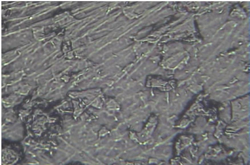
**Figure 2: Self-organization of resveratrol in the xanthan gum (0.25%) and a ratio of core: shell 1: 3 at a magnification of 2830 times.**
