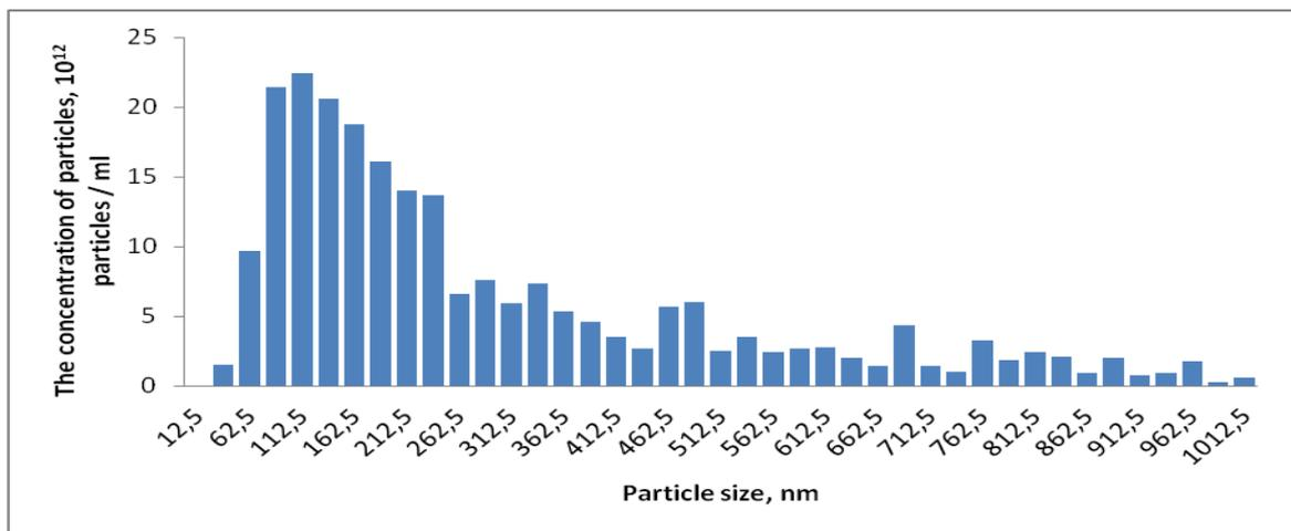
Figure 4: Particle size distribution in a sample of nanocapsules of resveratrol in the xanthan gum (ratio of core: shell is 5: 1)
